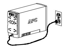
• The Back-UPS charges the internal battery any time it is connected to a wall outlet.
